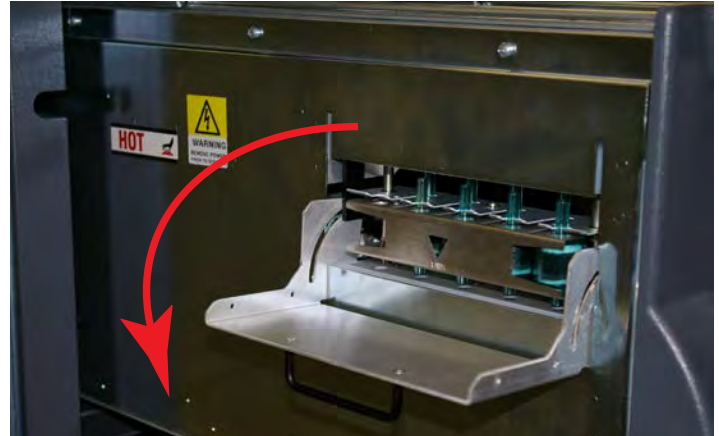
Figure 5-5. Pyrolyzer Filter Door
